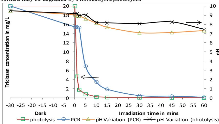
**Figure3: Time course profile for PCR and photolytic degradation of triclosan**
