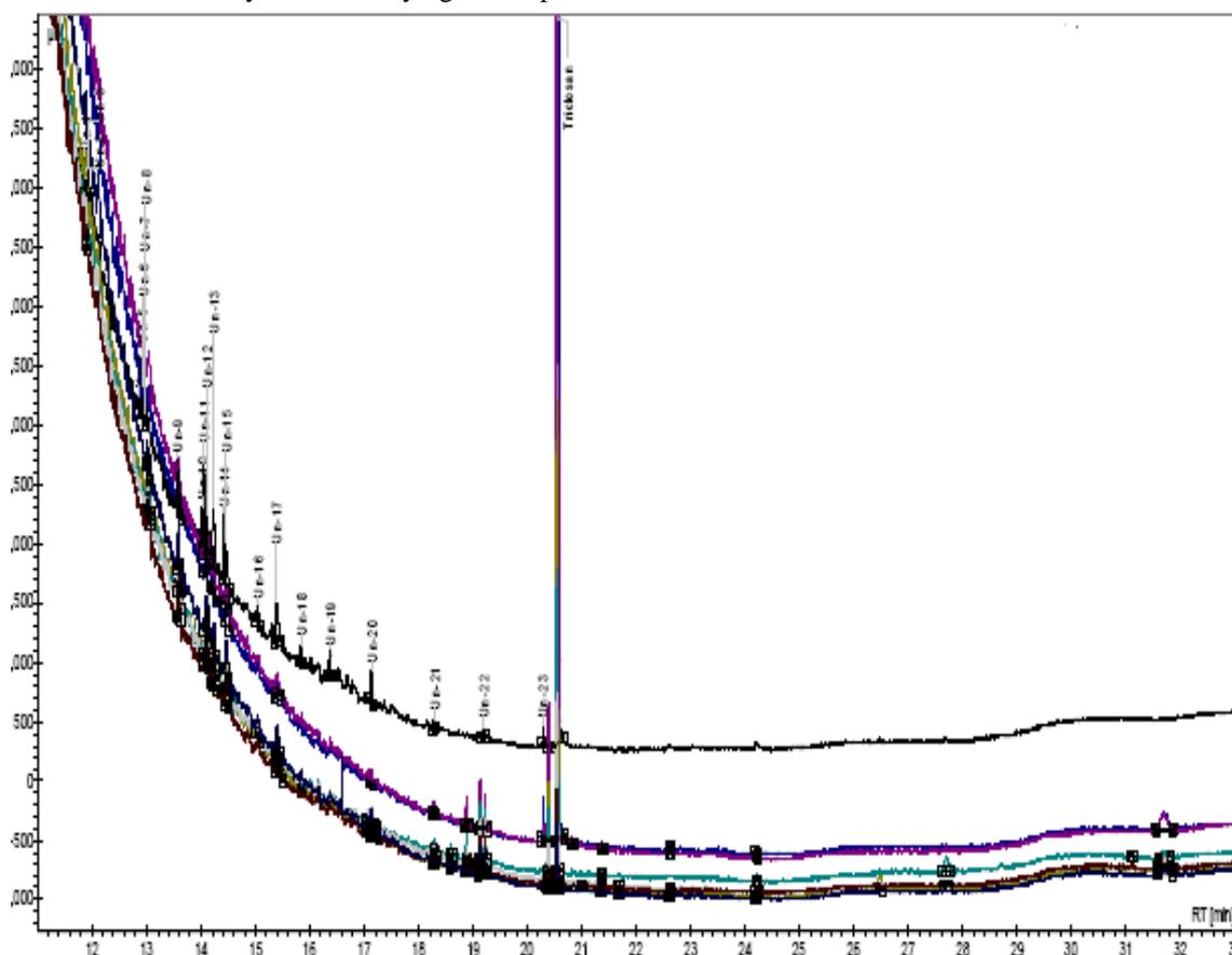
**Figure1: GC –FID chromatogram at different time points during PCR of Triclosan**
