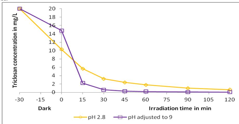
**Figure2: Time course profile for triclosan degradation at different pH**
