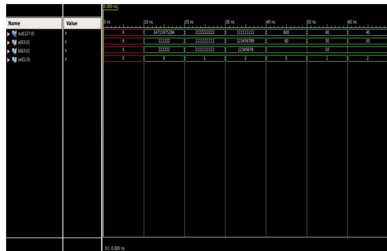
Fig :- Output of 64x64 Vedic Multiplier
