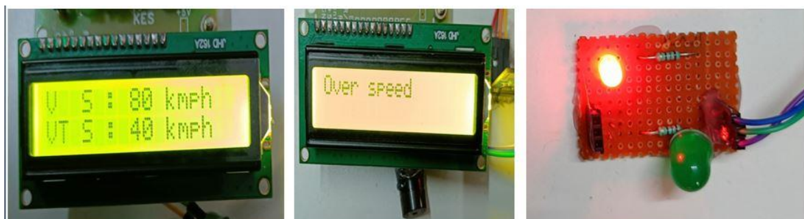
Figure 10 : Overspeed Detection and Alerting at School Zone
