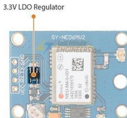
Fig 6: LDO Regulator in NEO-6M GPS module
